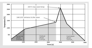
The total welding time, i.e., from room temperature up to the peak temperature of 265°C plus cooling, is a maximum of 10 minutes. The rise time to the required temperature is influenced by t he design of the product structure and the power of the preheating section of the soldering equipment. The temperature measurement point for soldering comes from the pin end on the top side of the PCB, which is recommended to be 2.4 to 3.2 mm thick.
